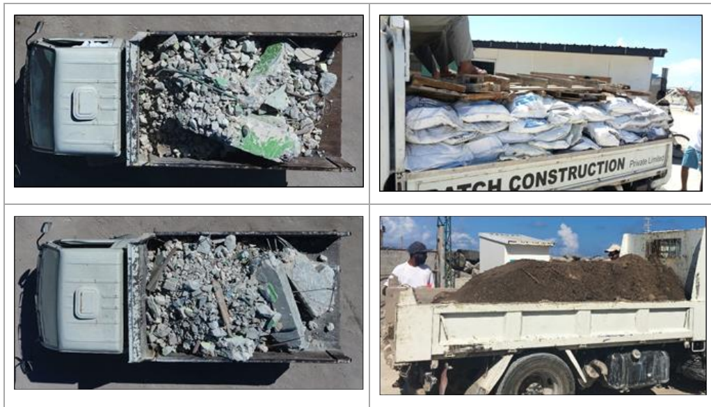
Figure 4: (a) Aerial view of a 2T truck containing concrete waste (b) Truck containing sand and rocks in polypropylene woven sacks with wooden pellets on top (c) Aerial view of a 2T truck containing concrete waste (d) Truck containing soil.
