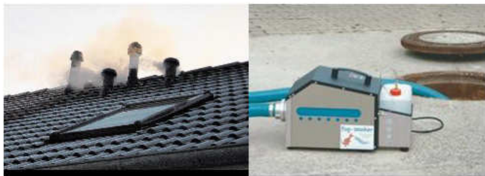
Figure 13 Detection of illegal connections
