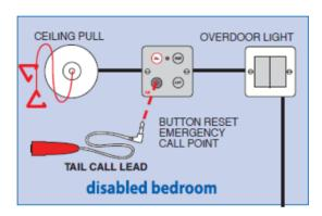
The master reset button of system's indicator panel-Nurse Control Panel should be able to enable or disable as this facility allows standard calls to be globally cancelled without the source of the call being investigated. The "Mute" button allows any standard calls on the system to be silenced but it leaves relevant indicator light(s) lit. Although a new call from a different call point will re-activate the sounder.
